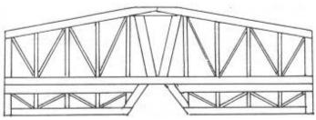
In the tail there is probably only one piece that has to have a little strength added. Most of the plans and kits I've seen just make the tail out of heavy wood. Sometimes it is sheeted. This type of stab often fails. The reason is that the tail isn't the whole story. There is a fuselage in there.
