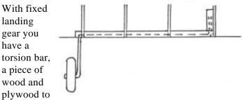
support it, the wire and the wheel. You want to make it into a retract. You've still got the wheel, most of the wire, some ply facing on the ribs to distribute load. You don't have those two pieces of torsion block on a retract, instead you've got the retract unit. These are pretty light. You've got a servo in the middle to run the retracts and you've got a slight difference of weight in the retracts themselves. To give you an example, the retracts on my 40 size Spitfire cost me 3.5 ounces.
