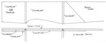
With the above construction, the plane comes in, bounces and breaks. There you have it - a fishead, lying on the flying field.
