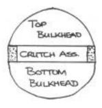
All the bulkheads are glued to this. Cut the bulkheads in half, glue all the bottom (or top) halves in place. Then you can set your wing saddle arrangement and stringers. Take it off the board, add the other side's pieces to finish it off.
