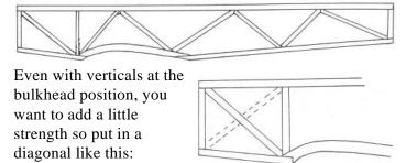
If you think about it, as you come into land, the motor wants to continue down and this diagonal, in compression, prevents the bay from parallelogramming. The triangle is doing its job. You can also put one going the other way.
