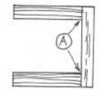
glue is not very strong in shear. There is not a lot of gluing surface. A good shear web in-between the spars is stronger, because the joint at "B" is not in shear and the glue is just there to hold it in place - not really much load on it.
