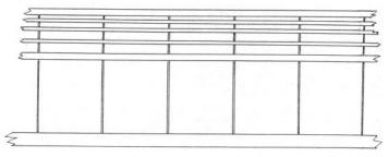
If you touch one wing tip on landing, the whole wing panel will try to parallelogram.
