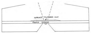
the fin down through the fuselage. Reinforce this with a small piece of spruce, tapered to avoid a stress riser.
