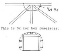
and you want to make it bulletproof, take 1/64" ply and gusset the inside of all joints. It adds hardly anything to the weight, but adds a tremendous amount of strength.
