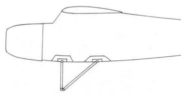
Like the trunnion block gear, this type also flexes out. Smaller diameter wire can be used than with the torsion bar landing gear of the wing. Use 1/8", 5/32", or 3/16" (for big planes), in wing torsion bar gear while 3/32" or 1/8" will work with this type of fuselage gear. There are all sorts of variations on this and different ways of doing it, but this is a pretty good landing gear.
